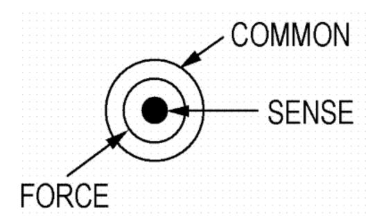
In the SMU case, the GUARD line is usually kept floating, since it maintains the same potential as the FORCE line in order to prevent the leakage currents. However, in the GND unit case there is no GUARD, only FORCE and SENSE. Therefore, it is impossible to connect the GND unit with the Agilent E5250A in the same manner as with a SMU.
